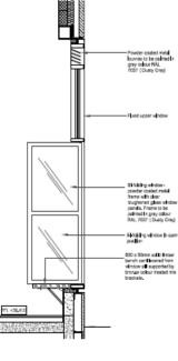
Typical Window Section (in open position) Scale 1:20 @ A1
